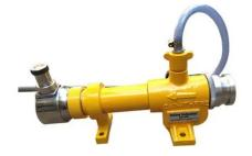
Portable Inline Inductors provide the means for accurate induction and mixing of foam concentrate into the water stream, for operation of foam branches and equipment. These Inline Inductors are matched to USAFE foam equipment such as LX, MX and HX branches and generators.
